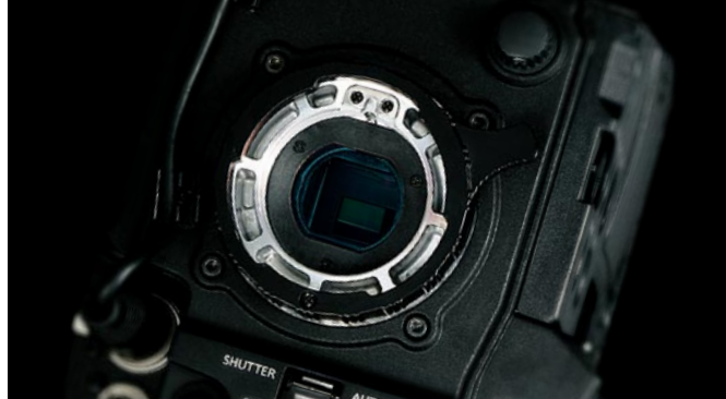
The 2/3-type bayonet mount interchangeable lens system
