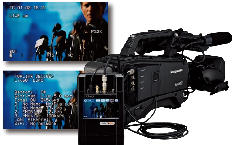
Example of a system with LiveU LU40 series. The uplink status is displayed on the viewfinder.
