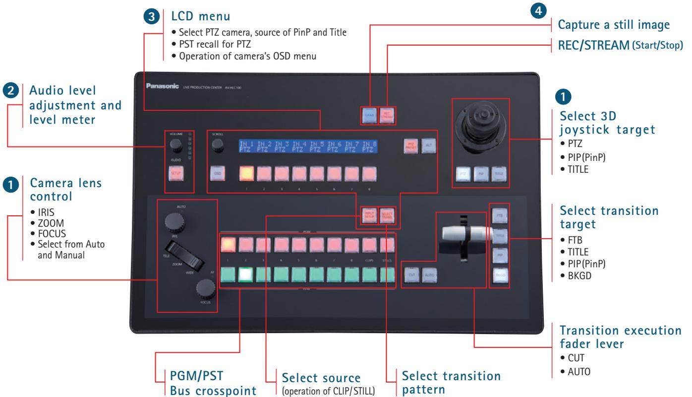
The extremely user-friendly panel includes buttons for various functions including camera control and switching, along with audio mixing. Up to eight video systems can be freely assigned to the crosspoint buttons, enabling them to be selected easily. With the capability to handle IP input and output, the AV-HLC100 also allows for live streaming and recording all over IP.
