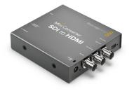
Now it's possible to convert from SDI to HDMI in all SD and HD formats up to 1080p60! Audio is embedded into the HDMI output and output separately as balanced analog or AES/EBU audio. Mini Converter SDI to HDMI is perfect for using HDMI televisions and video projectors as SDI monitors for all SD and HD formats, and when you don't need the extra cost of the Ultra HD model!
