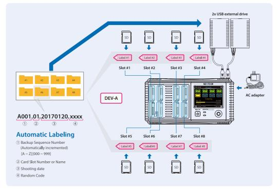
Assign camera man to the specific slot. Set the name of the camera man to the slot at the setup. The association between the camera and the backup folder is achieved through auto-labeling.
