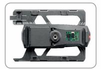
• iPad interface with built-in micro-processor ARM® Cortex®-A8 plus reliable Apple Certified tethered connection.
