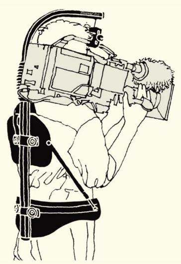
The EASYRIG portable camera support is ergonomically designed and reduces the static load on the neck and shoulder muscles, and transfers it down to the hips, the part of the body best designed to deal with it.
