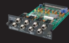
MY8-AD24 8 channel Analog Input Card
