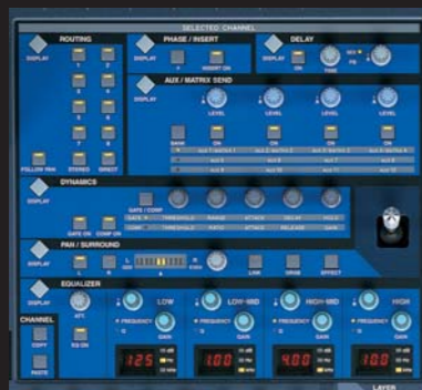
Selected Channel Section (DM2000VCM)
