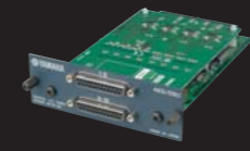
MY16-AE 16 channel AES/EBU format I/O
