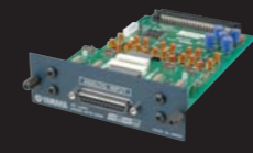
MY8-AD96 8 channel Analog Input Card
