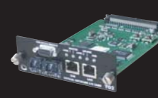
OPTOCORE YG2 16 channel Optocore I/O
