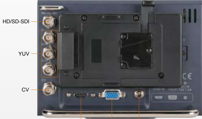
HD/SD-SDI YUV CV HDMI IN TALLY DC IN 12V 1.5A
