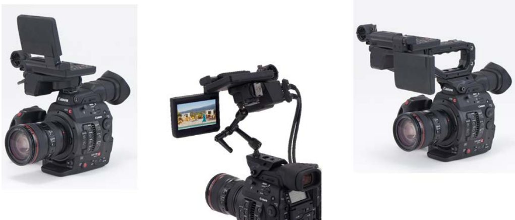
Figure 10 Showing on the right and left some of the options of mounting the LCD monitor, and in the center another alternative using a 3 rd -party mounting arm
