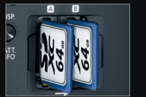
2 SDXC-compatible memory card slots
